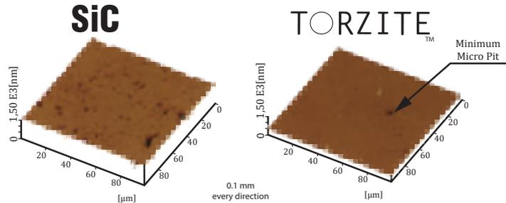
Torzite material features by minimization of micro-pores which wear out the fishing line. The mirror coating of Torzite material is much better than that of SiC guides.
