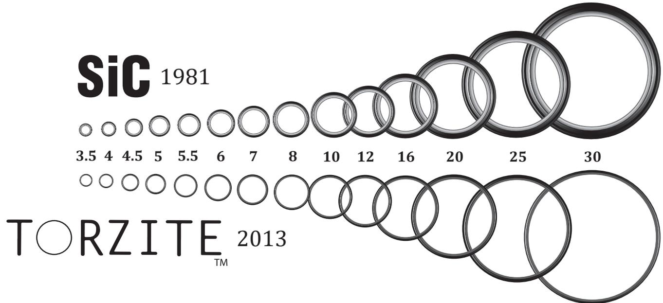
Due to incredible thinness of the new guide, its weight has been reduced and the inner diameter has been increased.
