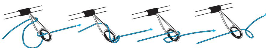
Loops that are formed during casting are being easily untangled because of the unique Tangle Free shape of the guide.
